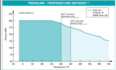
1. This chart displays the pressure-temperature ratings for the strainer's body material per ASME B16.1. Max temperature limits have been added for Quick-Open cover and Buna-N O-ring.
